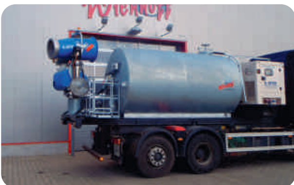
12.000l body with water cannon for binding dust
