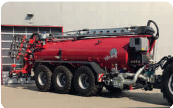
30.000l pump tank trailer + 8.50 m docking crane and 6 m Evers cultivator
