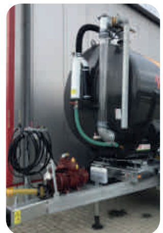
150 mm sight tube and hydraulic venting
