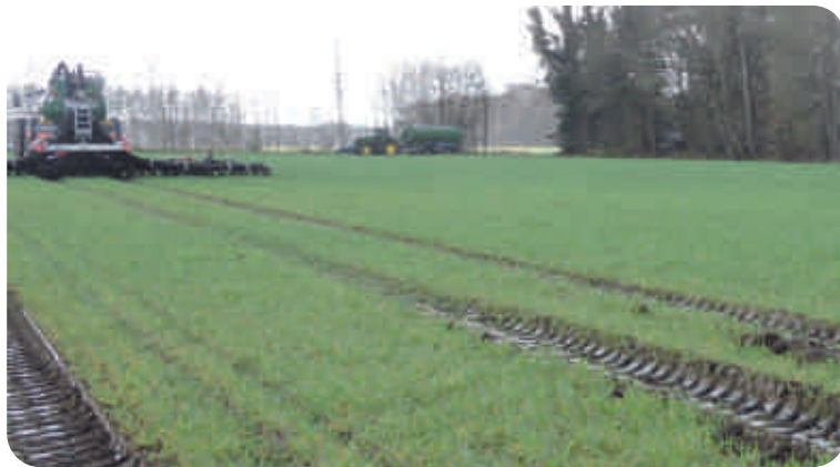
Change of the driving tracks after switching in the driving axle
