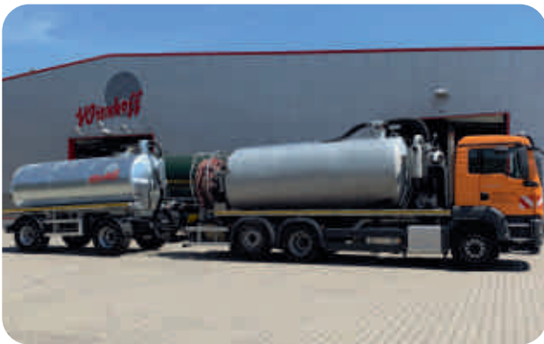
14.000l Abody + 14,000 l trailer with hose reel for suction from sewage treatment plants
