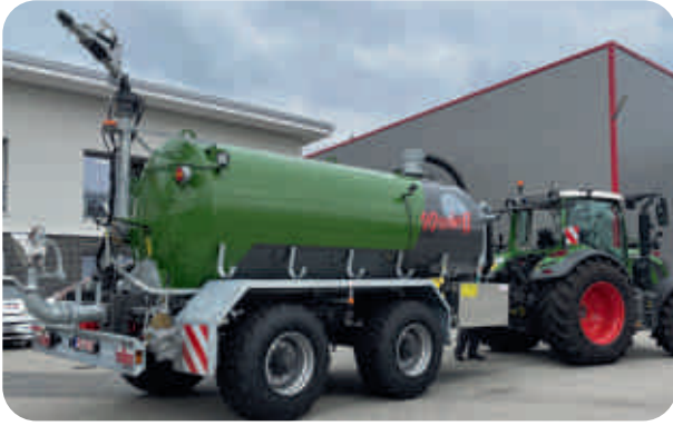
10.000l vacuum tank trailer + sprinkler
