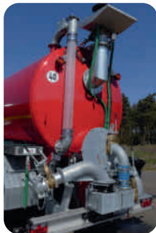
150 mm sight tube at rear with flushing and drip tray
