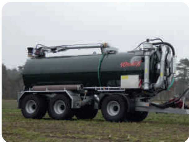
26.000l + + transfer pipe + double-articulated docking arm
