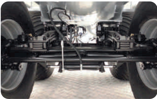
14-tonne bogie with parabolic suspension (mechanically offset by 2 positions)
