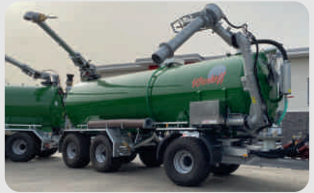
28.500l + + transfer pipe + double-articulated docking arm
