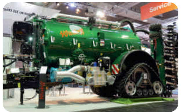
16,000 l pump tank trailer + driving axle + crawler track
