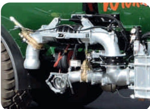
Docking arm, 1 joint, laterally swivelling with nicker
