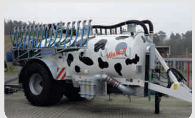
11.000l pump tank trailer + 12 m Bomech Speedy
