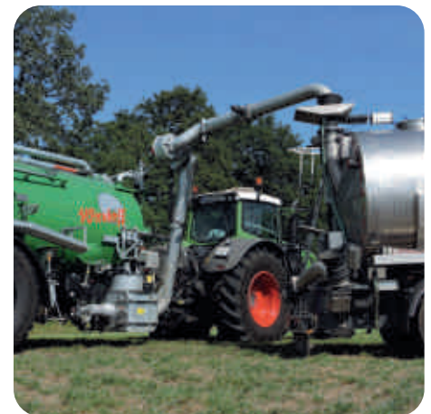
Suction spout + turbine + long docking ball
