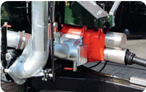
6.000l/min mech. rotary piston pump from Börger or Vogelsang
