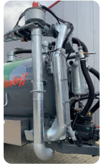
Suction spout + turbine, bent
