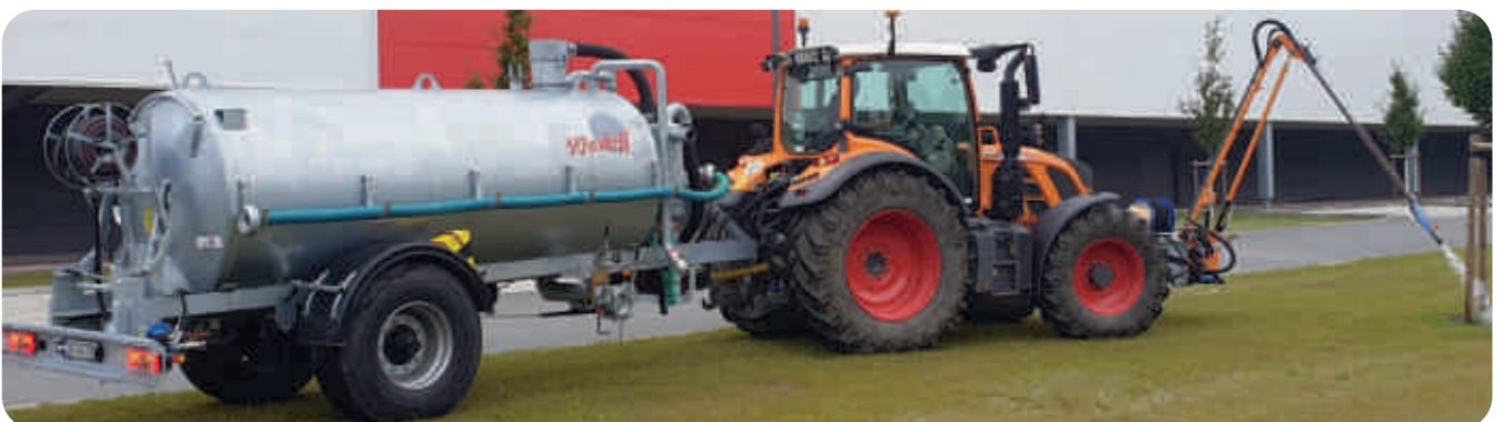
7.000l water drum + hose reel + centrifugal pump at rear
