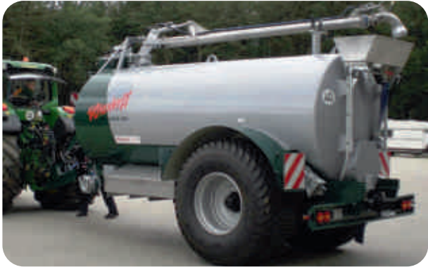
11.000l vacuum tank trailer for transferring liquid fertiliser
