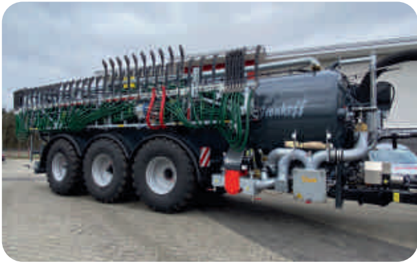
30.000l pump tank trailer + 30 m Vogelsang Slide
