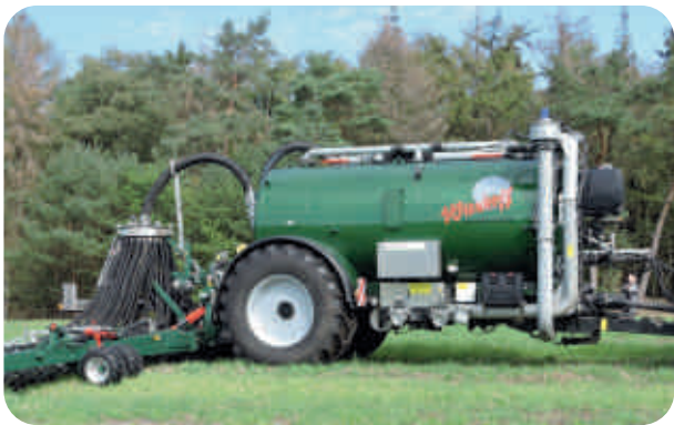
16.000l pump tank trailer + driving axle + 12 m Duport slitting device
