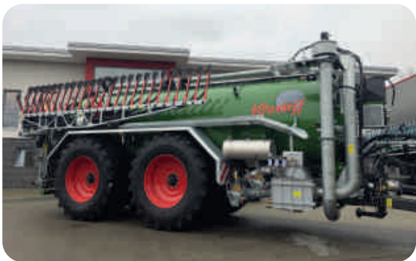
22.000l pump tank trailer + 900/60 R42 + 15 m BlackBird
