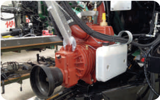
8.000-15.000l/min Battioni & Pagani vacuum compressor with oil top-up tank
