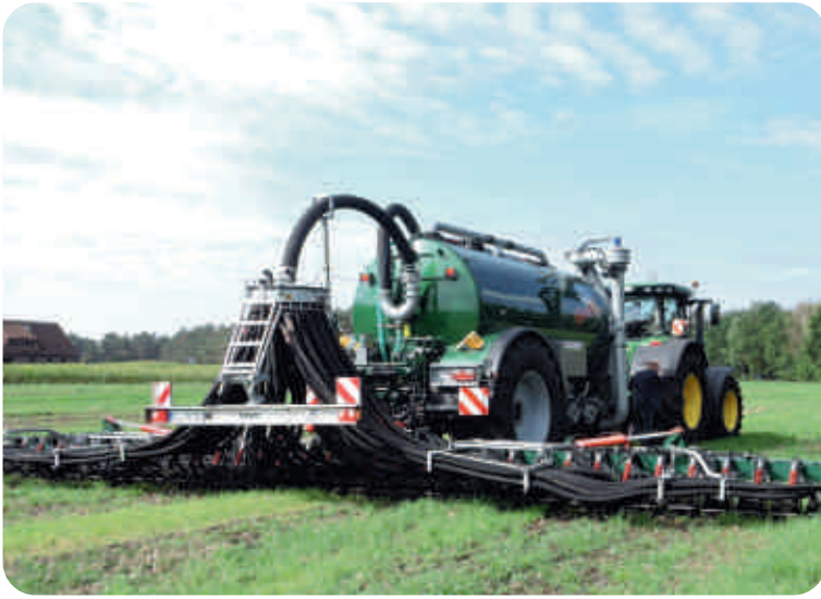
Rear view of single-axle trailer with slitting device
