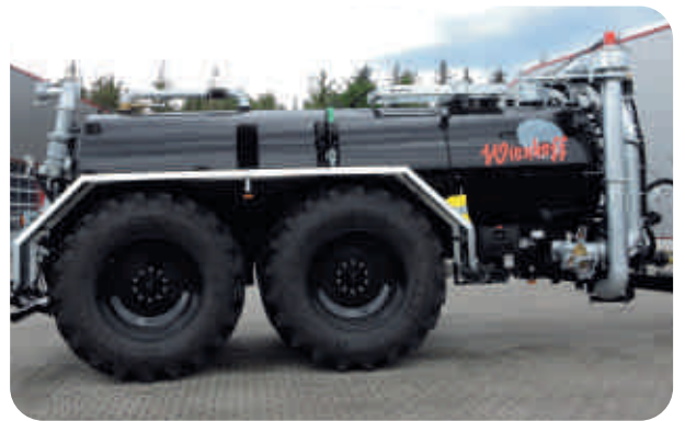
Specially fitted special construction frame for high steering angle with a maximum outer width of 3 m
