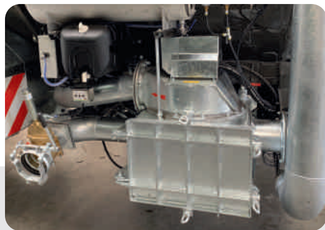
RotaCut RC 58H (12,000 l/min throughput) on large strainer box
