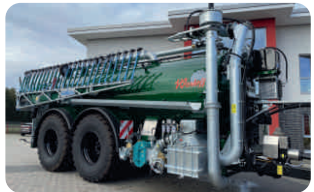
19.000l pump tank trailer + 15 m Bomech Farmer
