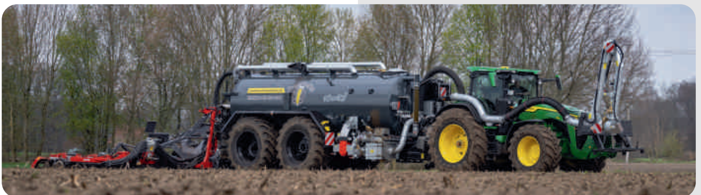
Tandem 28.000 l liquid manure trailer with driving axle + 13.50 m disc harrow
