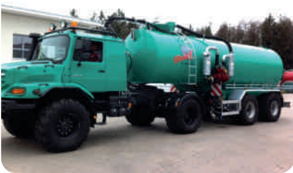
25.000l vacuum tank trailer tandem semitrailer for Mercedes Zetros
