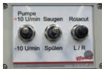
Auxiliary box for pump tank trailer with hydrostatic pump drive
