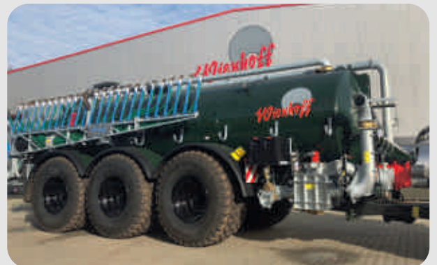
24.000l pump tank trailer + 15 m Bomech Farmer
