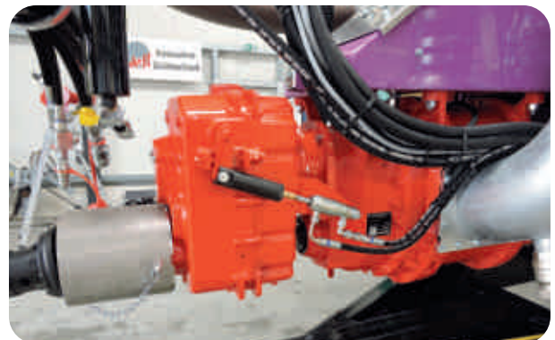
Rotary piston pump 9,000 l/min with two- or three-stage reduction gearbox from Börger or Vogelsang
