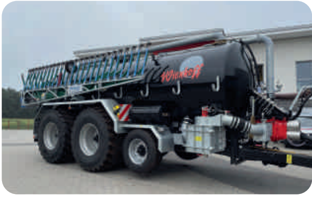
21.000l pump tank trailer + auxiliary axle + 15 m Bomech Farmer
