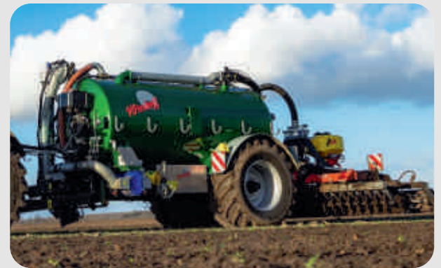
16.000l pump tank trailer + 6 m disc harrow
