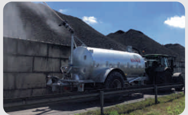
11.000l with sprinkler for watering coal heaps
