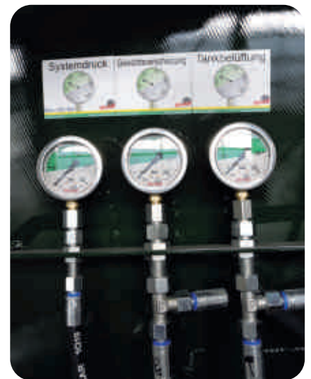
Hydraulic manometers on the front of the tank visually display the states of the hydraulic system to the driver
