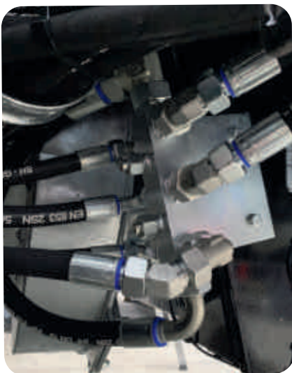
Large return collectors clear the way to your tractor's hydraulic oil tank
