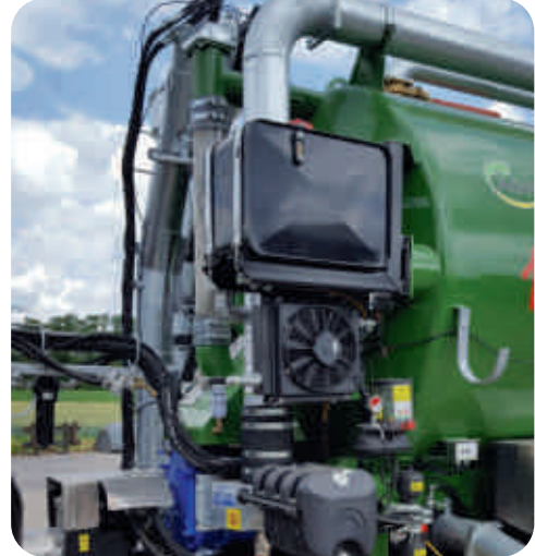
Axial piston variable displacement pump in a closed circuit for hydrostatic drive of the rotary piston pump
