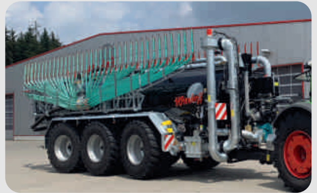
25.000l pump tank trailer + 19.50 m Wienhoff drag shoe
