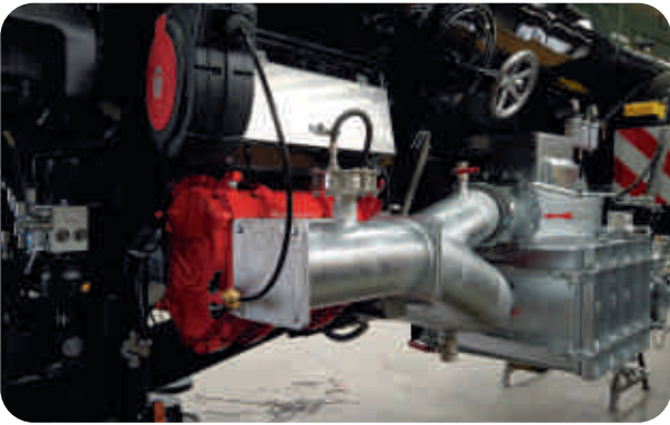
9.000l/min hydrostatically driven rotary piston pumps for controlling the exact spreading quantity
