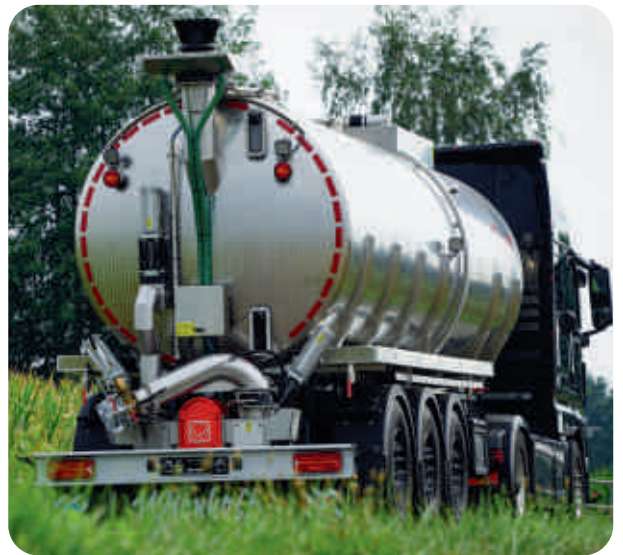
10" undocking hopper with drip tray
