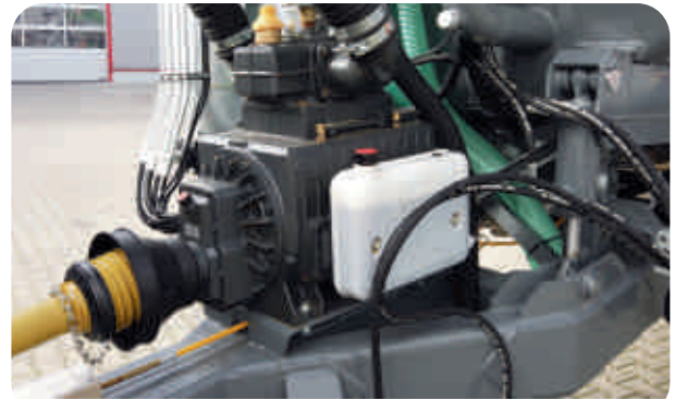
Water-cooled compressors for continuous operation
