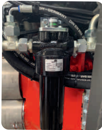
Preliminary pressure filters with display of the degree of soiling prevent dirt in our hydraulic system
