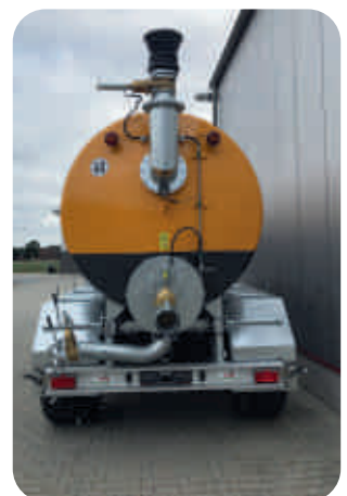
Additional LED lighting, 10" docking hopper pipe with 8" rubber hopper
