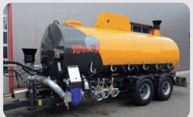
20.000l valveless filling and emptying
